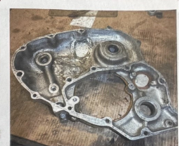
Note the alloy welded repairs, probably due to damage caused when it was thrown into a skip
