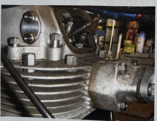
Setting the valve clearances – familiar to any Norton heavyweight twin owner
