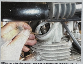
Setting the valve clearances – familiar to any Norton heavyweight twin owner
