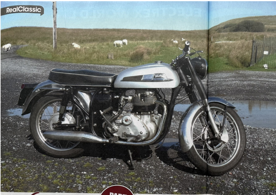
Part of the appeal of unit construction engines is that it's easier to make them compact with no separate gearbox. Observe the gap behind the engine in its featherbed home
