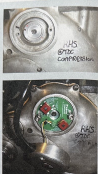
Timing marks added. Points would have been used originally
