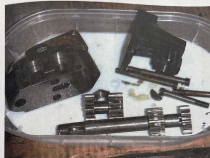
Oil pump stripped for inspection. It was reassembled using some readily available new components
